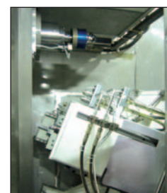
Spannvorrichtung in gekippter Bearbeitungsposition Clamping fixture in tilted machining position
