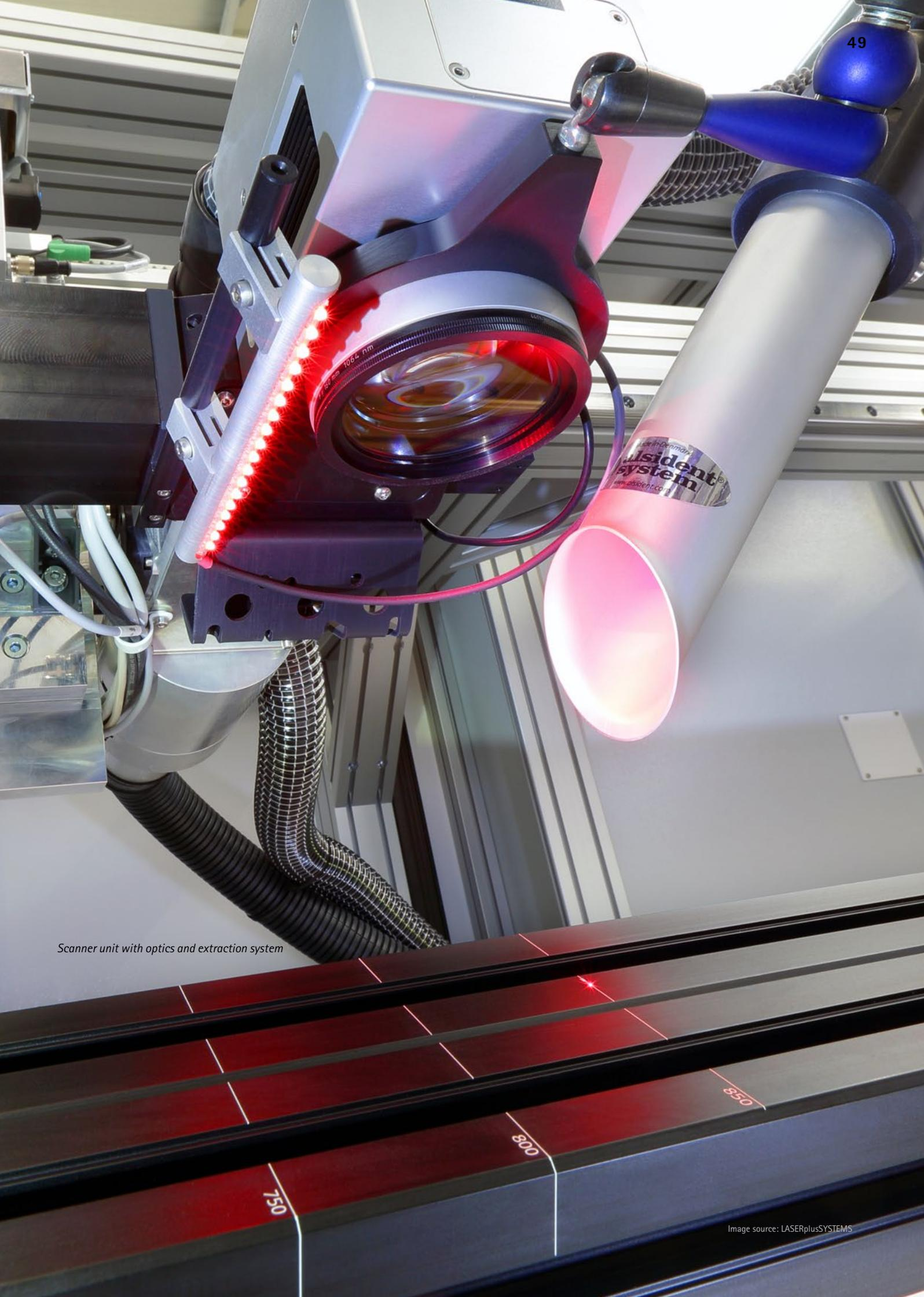
Scanner unit with optics and extraction system
